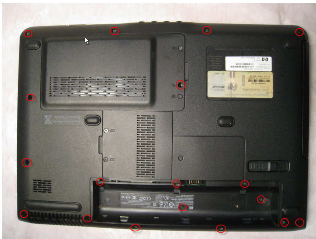
Remove palmrest and keyboard screws.
