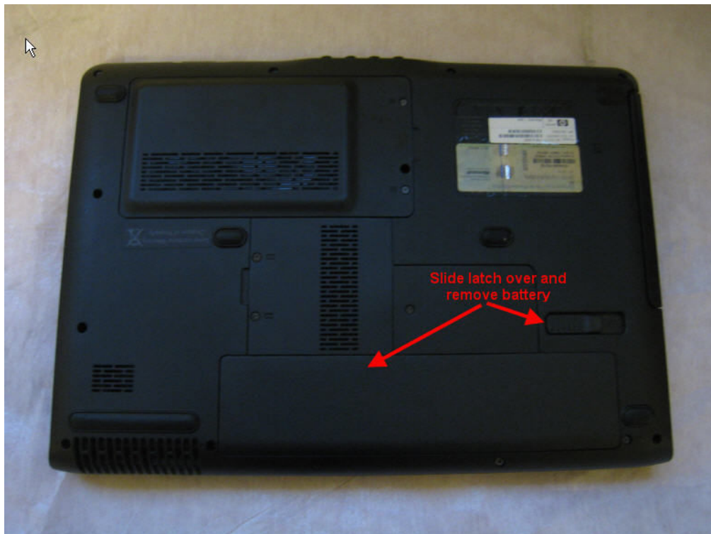
Slide hatch over and Remove battery.
